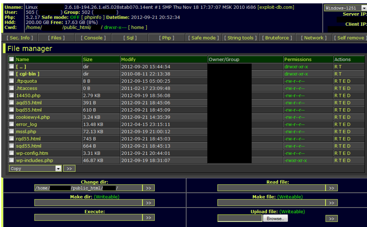
Figure 1 – PHP-based application for administering a compromised Web server
